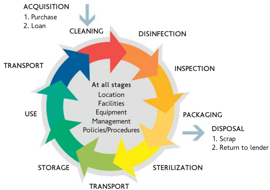
Figure 3.3.2. The cycle of decontamination of a reusable surgical instrument
